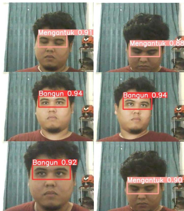
Figure 12. Detection of the state of driver's eyes using the custom YOLO V5 model
