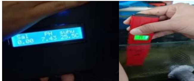
Figure 4. pH and pH Sensor Testing Meters
