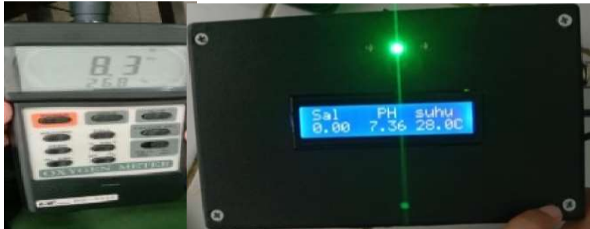
Figure 6. DS18B20 temperature sensor testing and DO/Temperature measuring instruments
