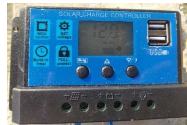
Gambar 5. Solar Charger Controller
