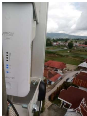
Gambar 11. Rocket Prism 5AC Dipasang ke Antenna Sectoral
