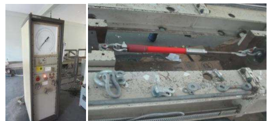
Gambar 15. Pelaksanaan Uji Tarik Temporary Insulator
